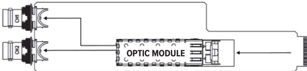
*Figure 13. Sample Camera Side Sync Card Signal Flow.*
