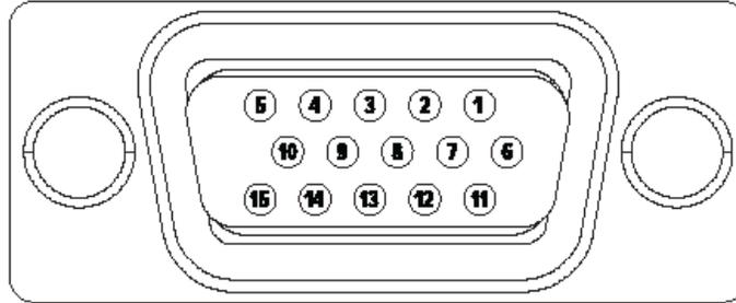
Figure 16. Data Card Cable Connector (Rear View).
