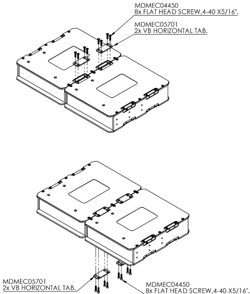
*Figure 22. Single VB Box Horizontal Rack Mounting.*
