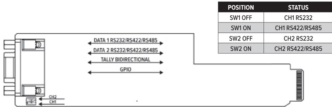
Figure 14. Sample Data Card Signal Flow (2 Bidirectional RS-232/RS-422/RS48, 1 Bidirectional Tally, 1 Bidirectional GPIO).
