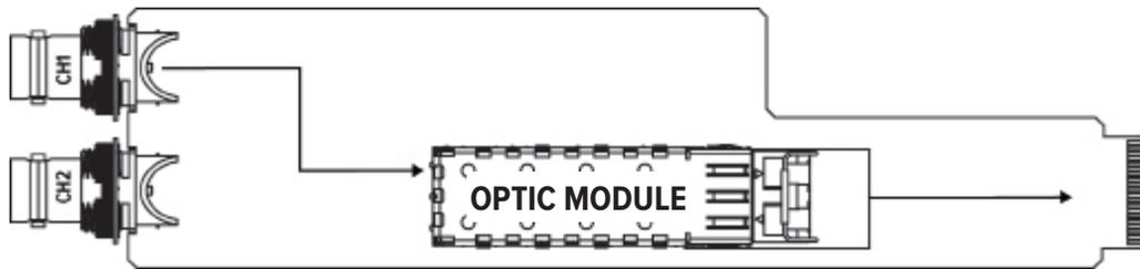
*Figure 12. Sample Base Side Sync Card Signal Flow.*
