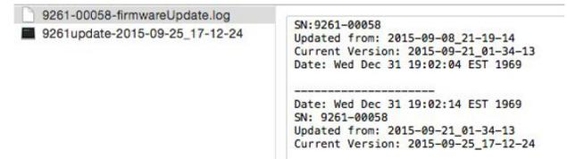
8. If more than one unit is upgraded using the same USB media device, there will be a firmware update log for each unit. The naming scheme for the firmware update log is <SN>-firmwareUpdate.log
