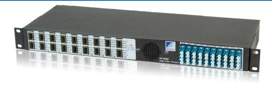
The VF-9000 is a 1RU, high density video fiber optic transport platform with 18 optical I/O (9 or 18 SFP Ports), it can be configured with up to 18 full size BNCs or 36 HD-BNCs. The system also supports up to 9 1GbE optical extensions, and provides the user with the option to handle SDI and LAN signals in one frame.
