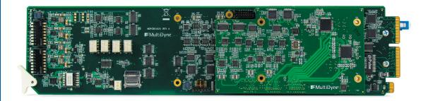
The OG-3600 series of modules for the openGear platform provides flexibility for all fiber transport needs. Signals are transported uncompressed and unprocessed from maximum signal integrity. Included signals are 3G HDSDI, audio, data, Ethernet, and reference, all compatible with the industry standard openGear platform offering SNMP management via Dashboard software.
