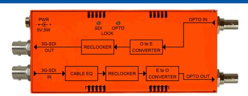
The NBX-TRX-3G-ST from MultiDyne provides a miniature solution to transmit and receive 3G/HD/SD-SDI signals over single-mode fiber optic cable using ST fiber optic connectors at distances up to 10km.
