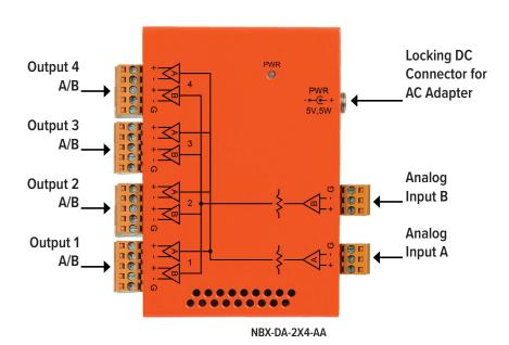
The NBX-DA-2X4-AA is an analog audio distribution amplifier designed for broadcast use. It provides up to 8 copies of the incoming balanced analog audio signal on pluggable terminal block connectors.
