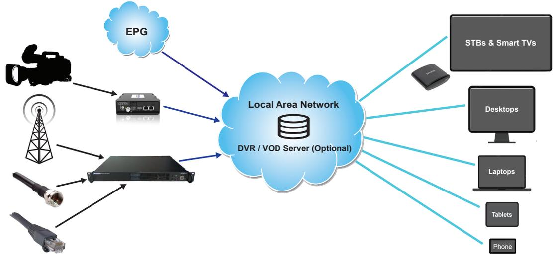
MultiDyne IPTV is a cost-effective solution that easily allows you to manage your live and file-based streams in your network or OTT content. The solution includes; Antenna (OTA) or Cable to IP converters; Niagara encoders and transcoders, Niagara IPTV management server, Android STBs apk, players for PCs, mobile devices or BYOD devices ( Amazon Fire, etc.)
