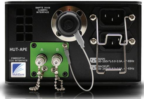
The HUT-APE system frees camera chains from the limitations of hybrid copper and fiber cabling permitting cameras to be separated from their CCUs by distances of over 10km using inexpensive, conventional single mode fiber. This has many advantages over SMPTE hybrid cable including:
