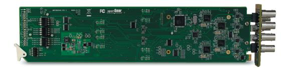
The HD-4000 series of modules for the openGear platform provides flexibility in how you handle your SDI signal transport. Capable of handling SDI rates from 5 Mb/sec all the way up to 3 Gb/sec uncompressed, these cards will automatically detect the incoming signal and give you full control over reclocking and routing.
