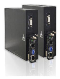
The FMX220-10GC-TS is a copper to fiber 10G Ethernet media converter based on IEEE802.3an and IEEE802.3ae. With SNMP and Web-based management in the FMX220, the Network administrator can monitor, configure and control the activity of each card in the chassis. This converter uses Cat.6a/Cat 7 twisted pair cable as copper transmission media with RJ-45 and
